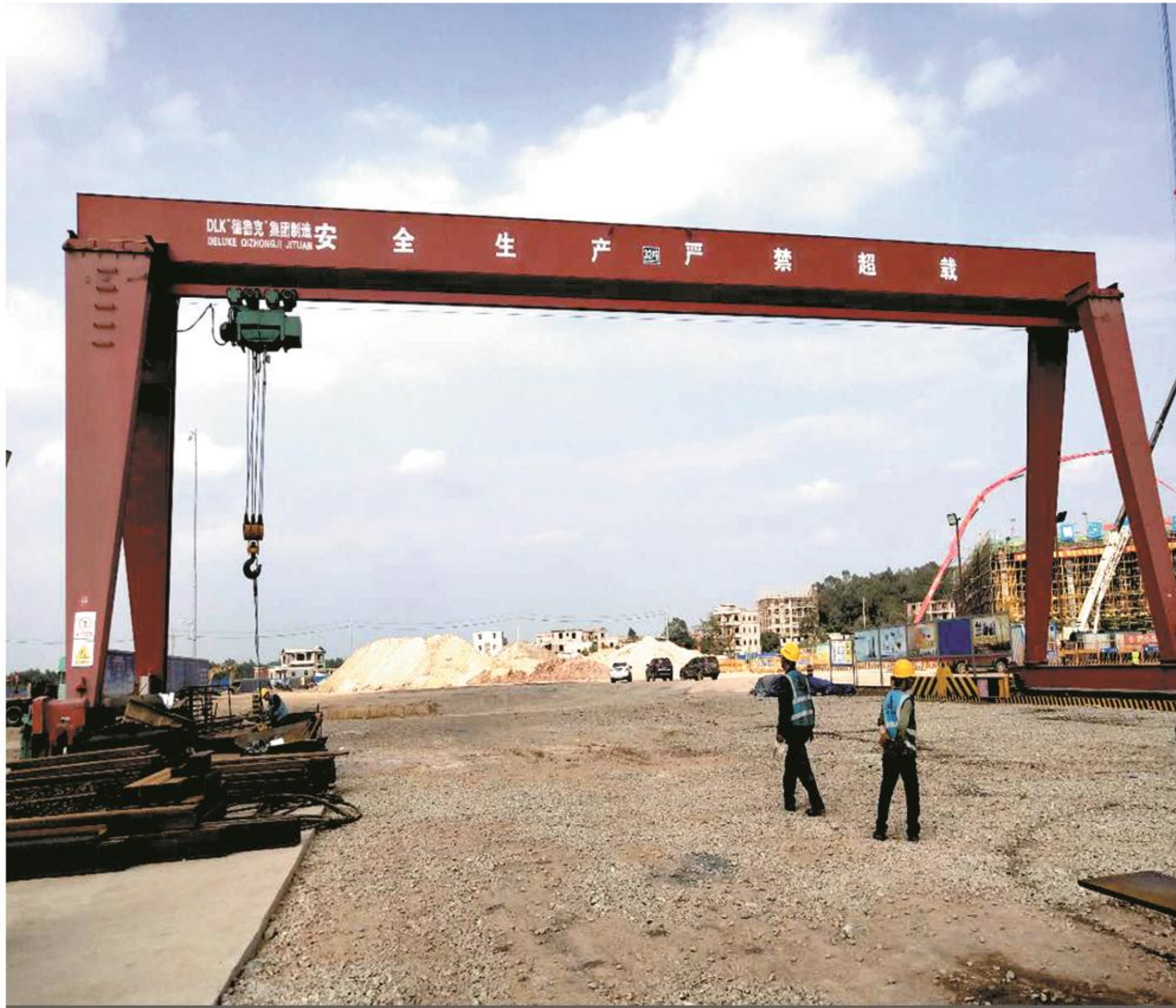
MH型电动葫芦门式起重机 MH electric hoist gantry crane 起重量 Lifting weight: 1-32 t 工作级别 Work level: A3
